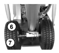
Fasten the wheel (7) on the base plate with the locking pin (6).
