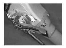
Slowly tighten the handle (1) of the reversing starter (2) until resistance is noticeable.
