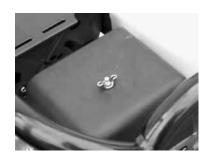
Remove the air filter insert from the air filter enclosure. Clean air filter insert as specified by the engine manufacturer if there is damage or if it is extremely dirty.
