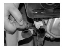
Screw the oil drain pipe (1) onto the engine drain valve and drain off the oil.
