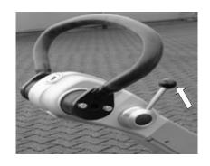
Turn the short-circuit button to the "0" – OFF position.
