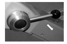
Slowly tighten the handle (1) of the reversing starter until resistance is noticeable.
