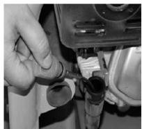
The correct oil level is between the min, and max, marks.
